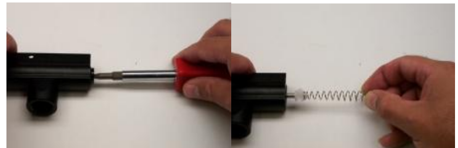
Diagram 1-4: Removing the volume chamber lug, cup seal return spring, and cup seal.
