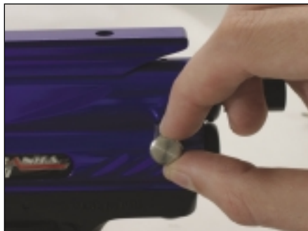
Figure 10. Remove field strip pin to begin disassembly.
