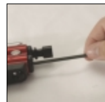
Figure 6. \frac{3}{16} " allen wrench is used to adjust velocity.
