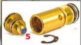
A leak from the back may be caused by an over pressurizing LPR this can be caused by damage to the internal face seal **5**. Replacing this portion of the LPR will return the pressure back to its normal range and will correct this leak.
