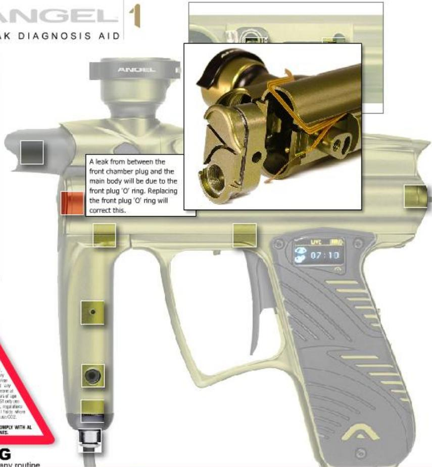
A leak from between the front chamber plug and the main body will be due to the front plug 'O' ring. Replacing the front plug 'O' ring will correct this.
