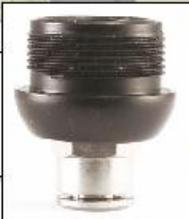
A leak from between the fore grip and the fore grip end cap will be caused by the end cap being loose, or the end cap 'O' ring being cut or damaged or out of its retention groove, replacing this 'O' ring and ensuring it is correctly located within its location groove will correct this.
