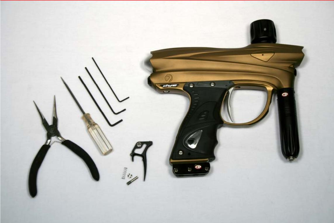
The following is a step by step guide to help you install a CP Sling Blade or Rake trigger into a DM6, DM7, or an ULTRALITE Grip Frame.
