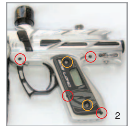
Open Trigger Frame
