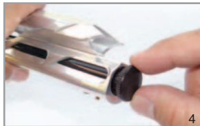
Remove Ram Sleeve Cap
