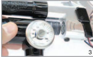
Slide Regulator Base from Body
