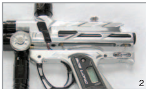
Separate Frame From Body
