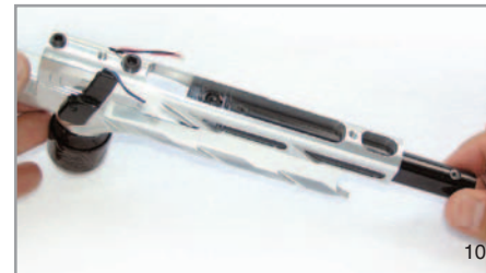
Remove Ram Sleeve from Rear
