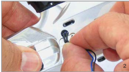
Remove Eye Sensors
