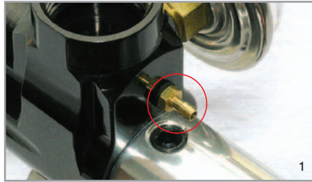
Remove Air Barb from ASA Block
