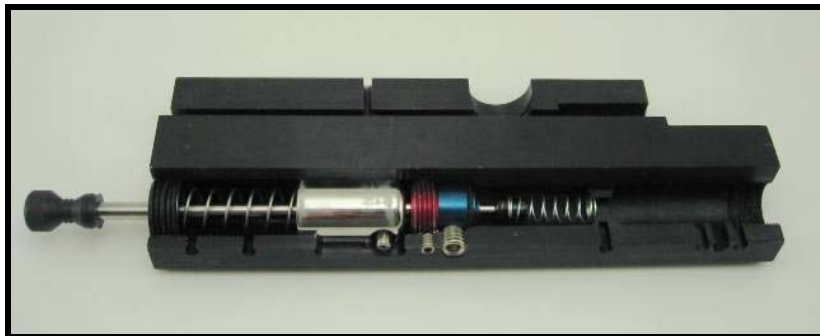
The light Valve Spring and heavier Main Spring force the valve open when not aired up.
