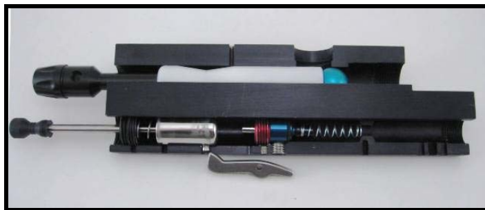
Sear Engaged, Bolt at rest, ball in chamber.
