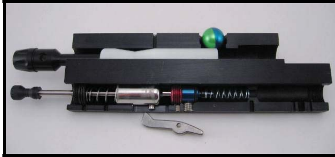
Marker being pumped – hammer and bolt traveling to the rear – ball ready to drop in breach.
