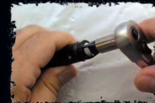
Loosen Valve Using 3/8" Socket
