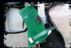
Flip Board, Remove Membrane
