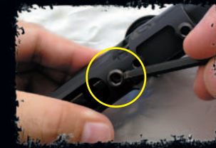
Remove Ram Sleeve Retaining Allen
