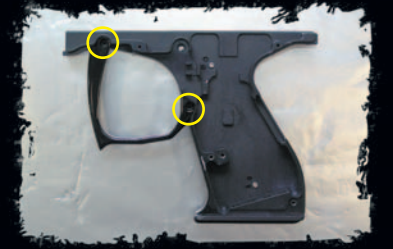
Remove Trigger Guard
