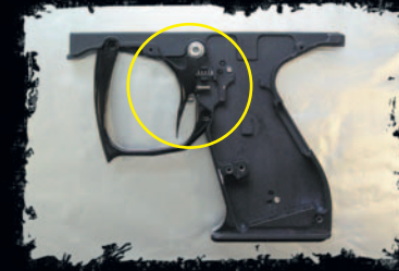
Remove Trigger & Spring
