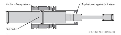
When the marker is fired, the trigger switch on the circuit board is pressed, telling the solenoid to switch the flow of air from the front of the cylinder to the rear of the cylinder. Air that enters the rear of the cylinder will push on the bolt sail, moving the bolt forward.
