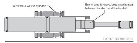
When the bolt moves forward, the tapered stem passes through a part called the Top Hat. The top hat is responsible for keeping air from escaping the supply chamber while the bolt is in the back position. When the bolt moves forward through the top hat, the tapered stem allows the air to pass, flow forward, and propel the ball.
