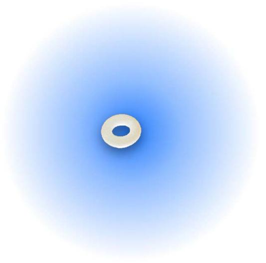
Found in the On/Off assembly the Teflon O-Ring opens and seals with every shot. Replace this o-ring if you can pull and hold the trigger and you still hear leaking out the barrel. This o-ring is not rubber but more like plastic. Do not dent or abuse it.
