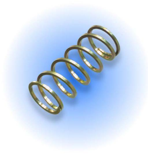
The Bolt Spring fits all AGD markers regardless of age or type. They are made from very special square wire so they don't fold inside themselves when collapsed. Replace your old springs when they sag below the front of the bolt. Special honed bolt springs come with Superbolts to prevent premature wear. One spring also comes in the Parts Kit. If you need any o-rings the kit is a good value.
