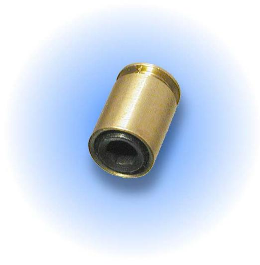
The Regulator Piston comes as an assembly. DO NOT take this apart. It has a built in blow off valve that will leak air if your marker becomes over pressurized. The blow off resets once your pressure goes back to normal. This safety feature is found exclusively in AGD markers. Replace the entire assembly if your marker is shooting at normal speeds and it still leaks out the back.
