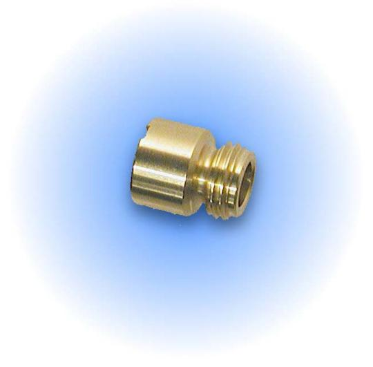
This item screws into the end of the Power Tube and is a precision part. It releases the air blast behind the ball in a controlled manner so the air hits the ball with low pressure to gently accelerate it out the barrel. Use a coin to tighten it up.
