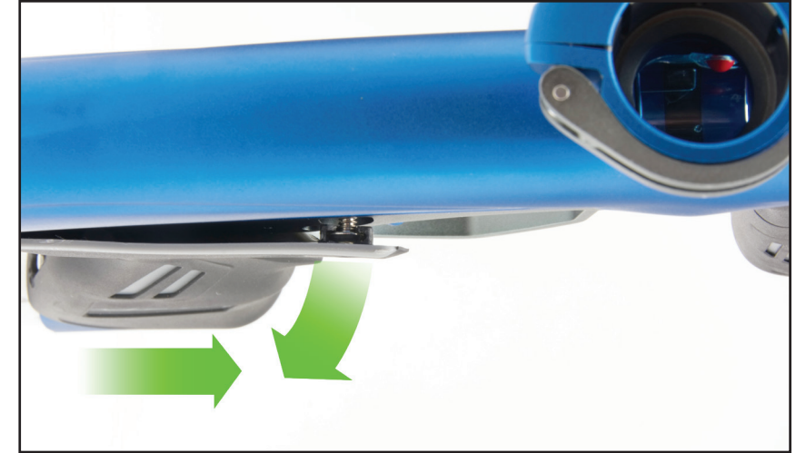
2. Pull the top of the grip away from the frame and forward to allow the upper rear locking hook to clear the frame.
