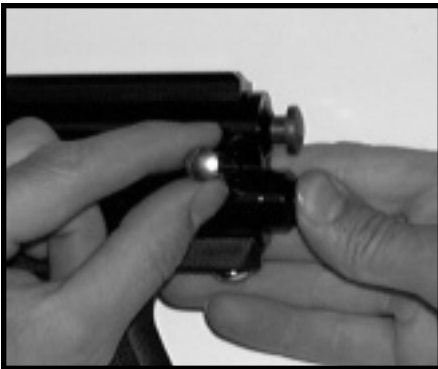
Figure 10 Remove field strip pin to begin disassembly.
