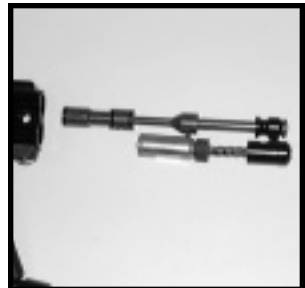
Figure 13 Bolt-hammer assembly removed.
