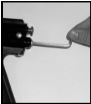
Figure 6 3/16" allen is used to adjust velocity.
