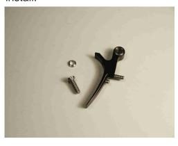
Stepped side of spacer should be facing towards the bearings.
