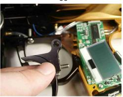
You should have your CP trigger with screw and spacer ready to install.
