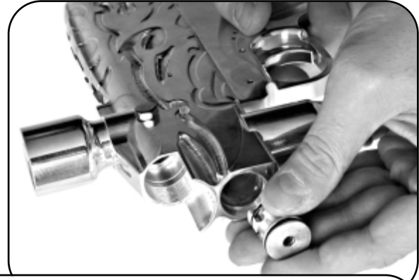
14. Pull out the AOC body (# 26), using AOC body extractor (# 78)* (insert the extractor's tip into the front whole of the body (# 26) press it downward and pull it out).
