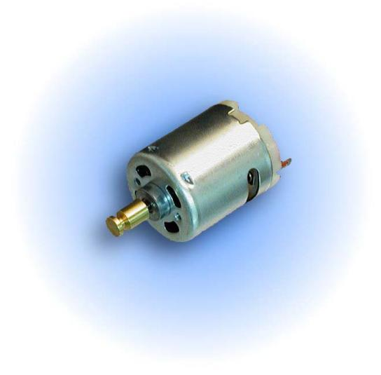
Motor comes with pulley assembled as a unit. Co33nnections must be soldered.
