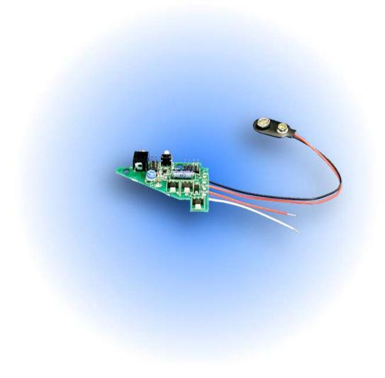
Board that controls the Warp. There are two springs under the board that make contact with the sensor; don't lose them.
