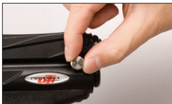
Figure 8. Remove field strip pin to begin disassembly.
