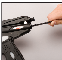
Figure 6. A \frac{3}{16} " allen wrench is used to adjust velocity.
