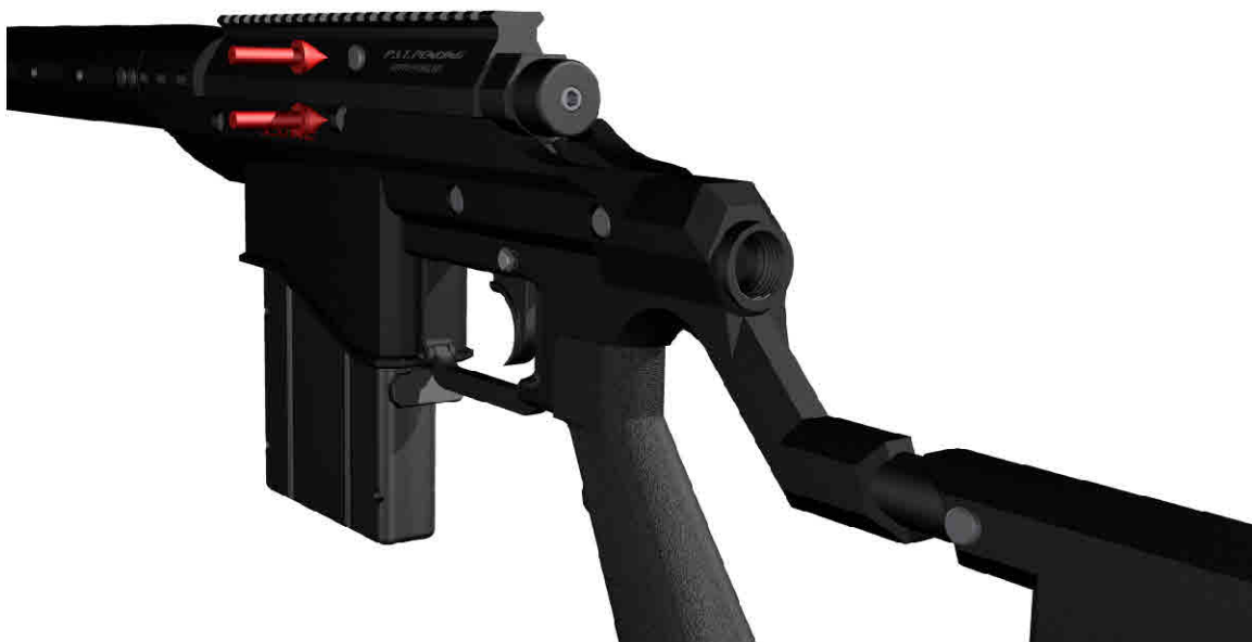
Figure 9: Engine Assembly Quick Removal Pins
