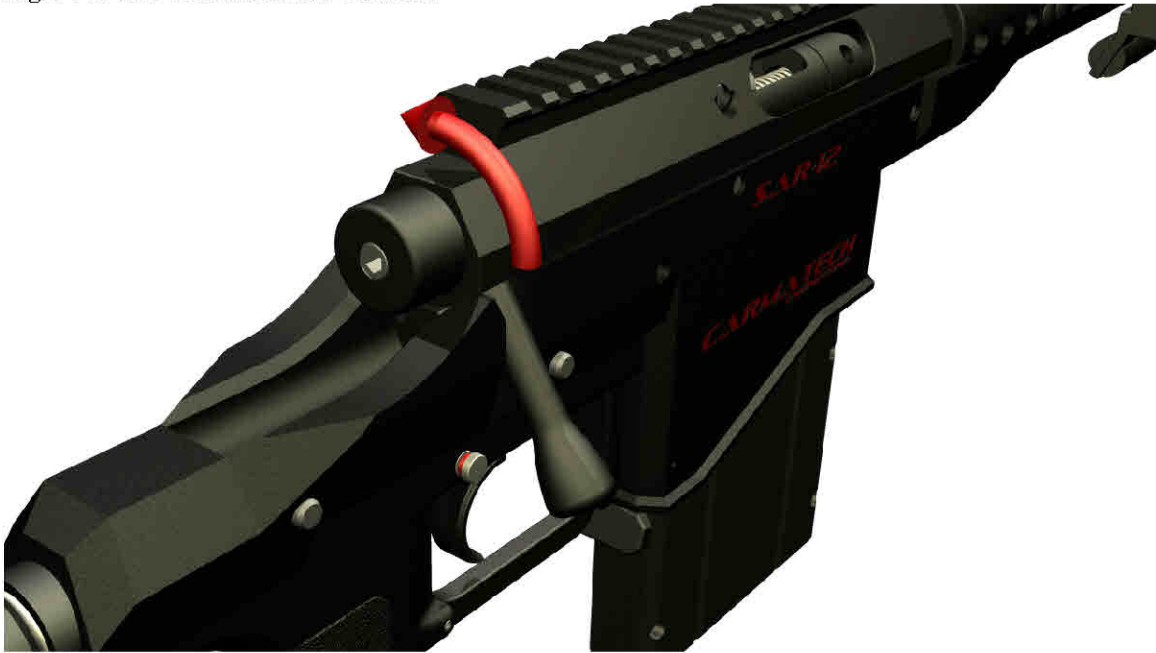
Figure 5: Bolt Action Handle Rotation
