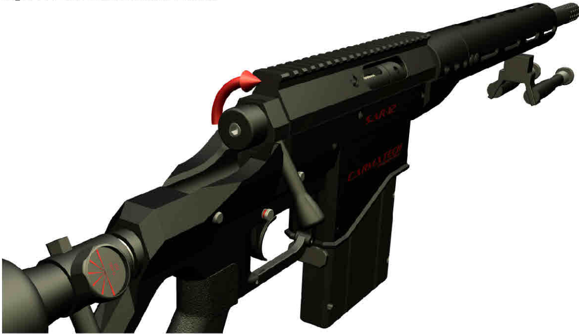
Figure 7: Bolt Action Handle Locked
