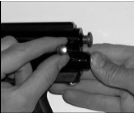
Figure 10 Remove field strip pin to begin disassembly.
