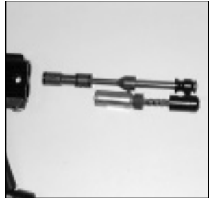
Figure 13 Bolt-hammer assembly removed.
