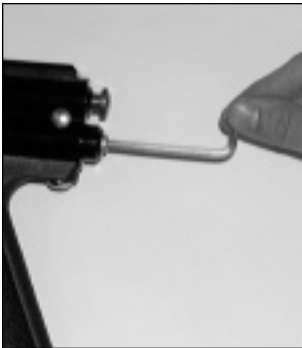
Figure 6 \frac{3}{16} " allen is used to adjust velocity.
