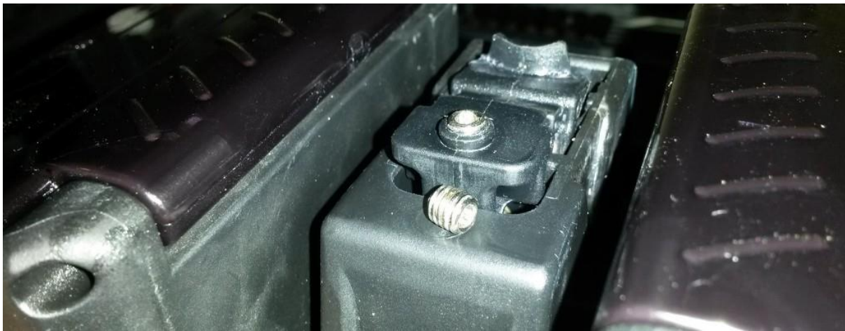
Box Rotor Stack Retaining Detent - Modified with set screw
