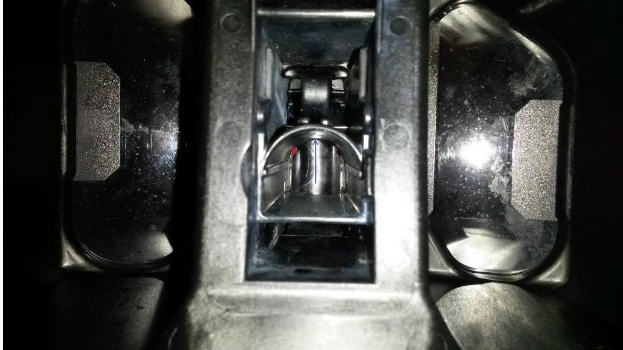
Image taken from within the Box Rotor showing that the Retaining Detent has been retracted all the way back and is not obstructing ball movement.
