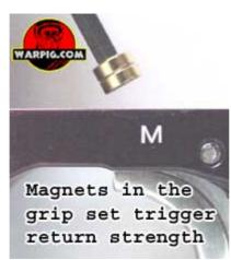
A magnet in the top of the trigger is attracted to powerful rare earth magnets stacked in the grip frame to provide trigger return. Unlike a trigger return spring, which provides more resistance the further the trigger is pulled, the E-Mag's trigger actually provides less resistance as the magnets move further apart, for a very unique feel. The weight of the trigger pull is adjusted by the number of magnets stacked in the grip frame.
