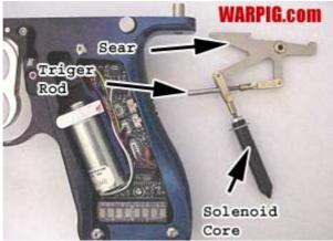
The E-Mag sear has an extra lobe, when compared to a normal 'Mag sear. A clevis pin attaches to this, allowing a solenoid to pull the sear. A solenoid is basically an electro magnet. It is made of a coil of wire that either pulls or repels a metallic
