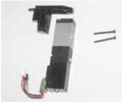
Solenoid removed from manifold
