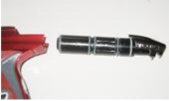
Firing assembly removed from body
