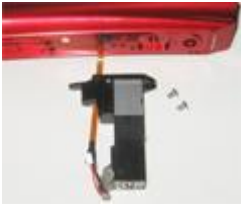
Solenoid manifold removed from body
