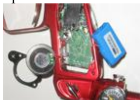
Speaker and battery removal
