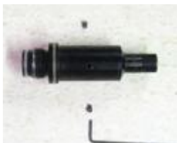
Dogbite set screws removed
