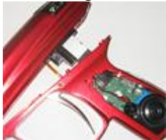
Inserting the solenoid into frame
