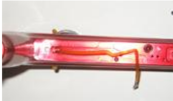
Both eyes threaded into the wiring canals
