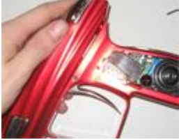
Aligning solenoid inside frame
