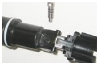
Quickstrip latch pin vent hole
