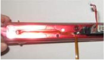
Body's eye ribbon retaining slot
