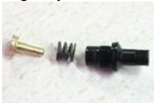
Reg piston and spring removed
