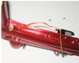
Threading the eyes into body wiring canals
