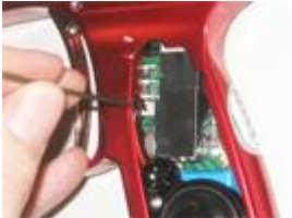
Solenoid connector reinstall
