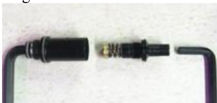
Reg body disassembled
