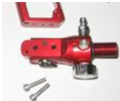
Bottomline screws and regulator removed
