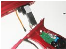
Threading the solenoid connector into frame
