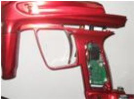
Gentle removal of the frame
