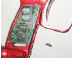
Board screws removed
