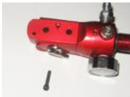
On/off knob retaining screw
